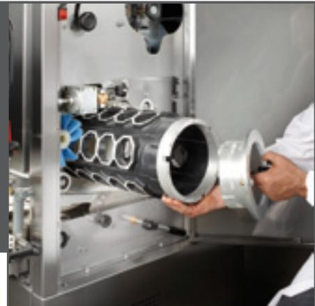
DINAMICA is produced in 3 different models, the DINAMICA 4, 5, or 6 pockets. Each model has different versions and the customer can choose one, two, or all the variables inside the same model. Different versions (factory set) can be modified later to meet the changing needs of the client, with the purchase and installation of a special kit of "changeover" pistons and the rounding drum.
