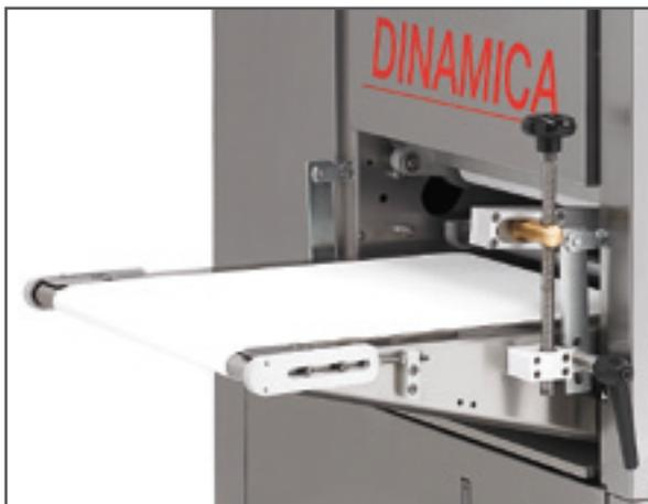
Solid and heavy duty out feed belt for hand panning (Standard).
