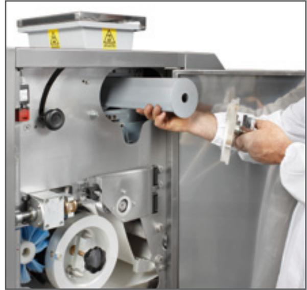
The special plastic material allow the machine to be OIL FREE. This feature provides a huge advantage to the baker, by reducing the time required for maintaining a clean machine, being a great money saver to rid the need for divider oil for machine operation. NO OIL, NO MESS, SAVES MONEY!
