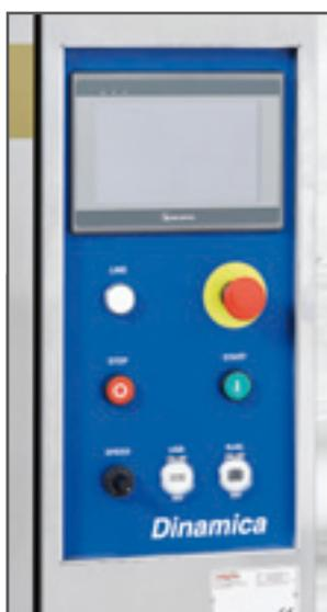
The panel also has a diagnostics screen to identify possible operational problems. Further, the panel can identify conflicts where the dough weight, the production speed, and, the overall machine speed are non-synchronous, mechanically or through the potentiometer.
